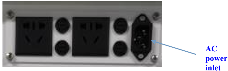
Figure 5-1 AC power inlet
